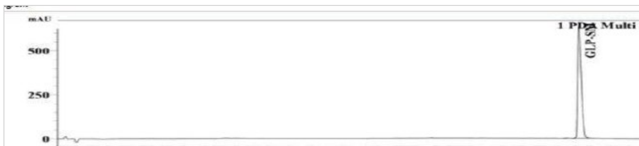
Semaglutide 10mg - VRL-SEM-2605: UV Chromatogram
